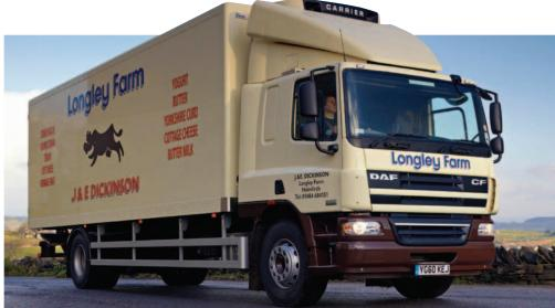
Since their runs involve nights away, both trucks were specified with the DAF sleeper cab, and Paneltex of Hull built and fitted the 53 cubic metre fridge bodies to each of the trucks' 6.9 metre wheelbase
