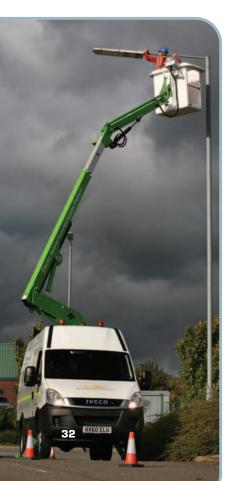
PJ Hire Services has taken delivery of the first Euro 5 van in the UK to be mounted with a hybrid Versalift mobile access platform that can operate without the vehicle's engine running.
